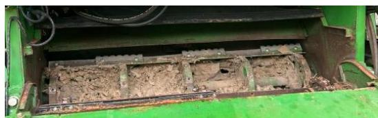
**STEP 3: CLEAN THE DIRT IMPREGNATED ON THE FLANGES AND CYLINDER**
