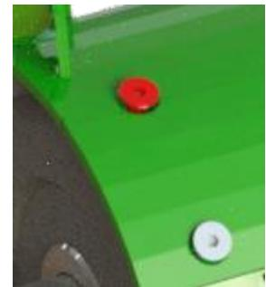
**STEP 16: REPEAT STEPS 14 AND 15 ON THE LAST COVER. WITH ALL THE SCREWS PRE-POSITIONED, START THE FINAL TIGHTENING THROUGH THE COVER WITH 04 HOLES APPLYING 72 Nm, ALWAYS STARTING WITH THE CENTRAL HOLES OF EACH COVER**
